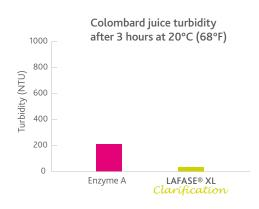
The clarification kinetics of Chardonnay and Colombard juice samples (South Africa) were monitored in 1 litre Imhoff sedimentation cones. Enzyme dosages: Chardonnay – 3 mL/hL (due to very high turbidity of the juice) and Colombard 1 mL/hL. The initial turbidity measurement was >1000 NTU. LAFASE® XL CLARIFICATION showed the lowest turbidity after 3 hours of settling at 20°C (68°F).
