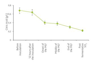
Figure 3. Evolution of the citric acid in a Chardonnay wine inoculated after the end of AF with LACTOENOS<sup>®</sup> 350 PREAC. Wine parameters before the bacterial addition: ETHANOL = 13.2% vol., pH = 3.3, L-MALIC ACID = 2.4 g/L, CITRIC ACID = 0.68 g/L.
