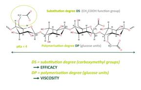
Figure 2. Sodium Carboxymethylcellulose molecule.
